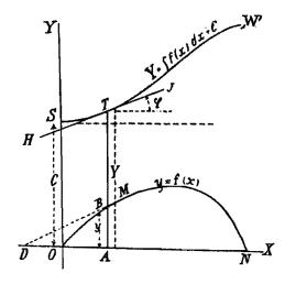
FIGURE 5 The use of the integraph for integration
